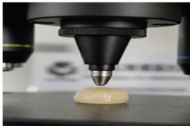
Figura 2 Aplikimi i testuesit Vickers mbi mostrën. Figure 2 Application of the Vickers Hardness Tester on the Specimen.
